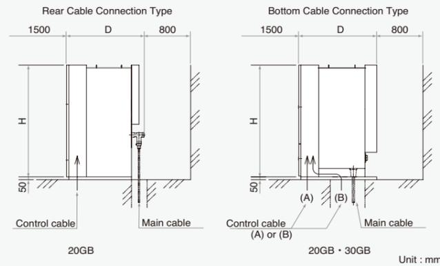
Fig.3 Switchgear Alignment
