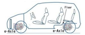
Due to its thinness, the MEIDEN e-Axle enables a layout of a three-row-seat when it is placed in the rear section of a vehicle
