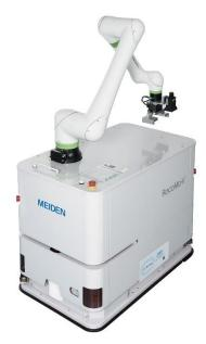
The robot's load capacity is 10 kilograms more than the previous model, but the exterior size of the AGV is the same. This allows the AGV, which is capable of traveling omnidirectionally, to travel in a stable manner on a path as narrow as 800 millimeters wide.
