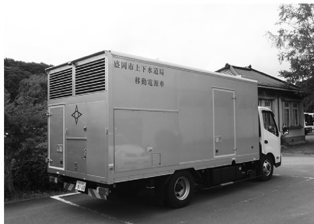
Fig. 6 Mobile Power Generating System at the Yonai WPC in Morioka City
