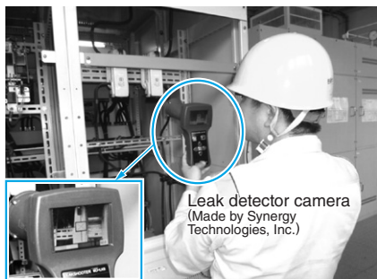
(b) A view of diagnosis by a corona detector with a camera
