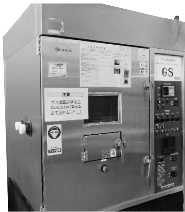
Fig. 10 Gas Corrosion Testing Machine
