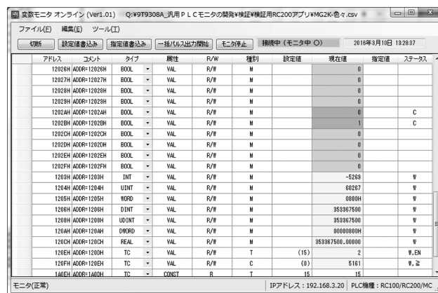
Fig. 12 Screen of General-Purpose PLC Monitor in the Middle of Monitoring
