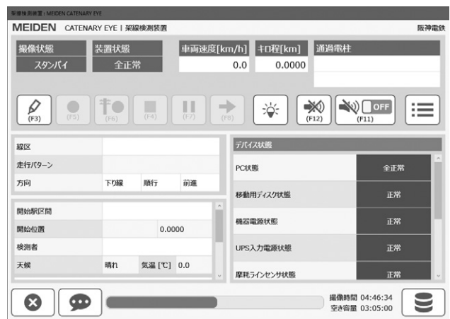
Fig. 5 Display Screen of On-Board Equipment inside Train
