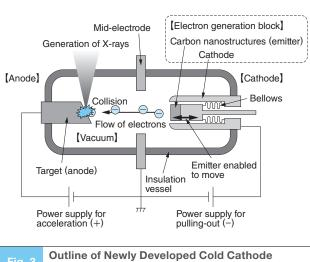
Fig. 3 X-ray Tube The newly developed cold cathode X-ray tube is devised to have
