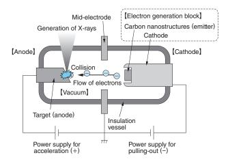
Fig. 2 Outline of Cold Cathode X-ray Tube
