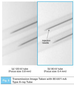
When the focus size is reduced, a fine object like a needle can be recognized clearly.
