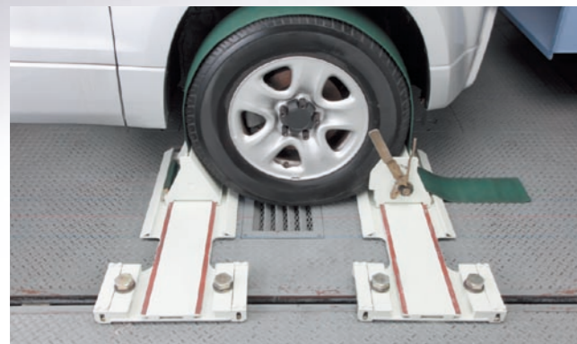
① Tire restrain type (Exclusively used for 2WD) Non-drive wheel is tied down by belt.
