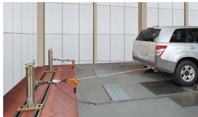
② 4-point pole-chain type (For 4WD) Test vehicle is restrained from the front and rear directions.
