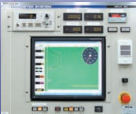
Driver's aid Driver's aid instructs motorcycle speed based on speed profile of each test mode.
