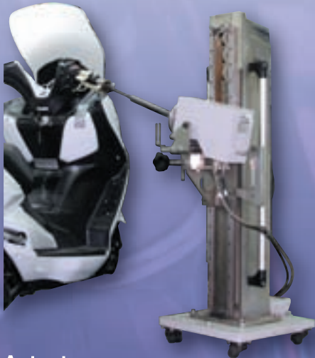
Actuator Speed, throttle opening, intake air pressure are controlled through throttle operation.
