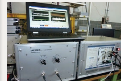
A device for measuring partial discharge using electromagnetic waves
