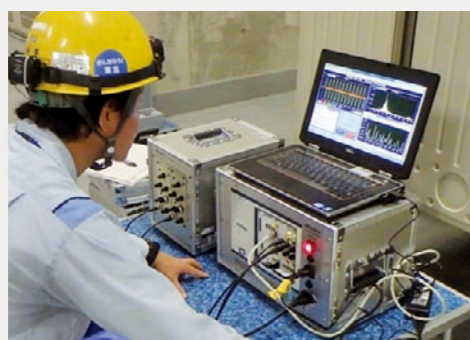
Partial discharge measuring unit by the use of AE sensor
