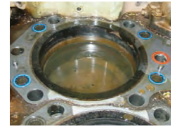
Intrusion of cooling water caused by deterioration in the pack
