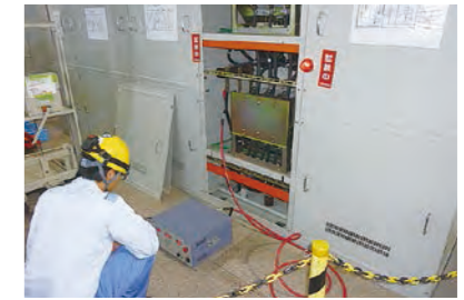
Diagnosis of power cable insulation
