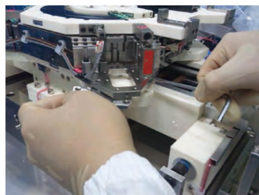
Exposure stage mechanism repair and refurbish
