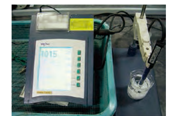
Analysis of equivalent salinity adhesion amount by conductivity meter
