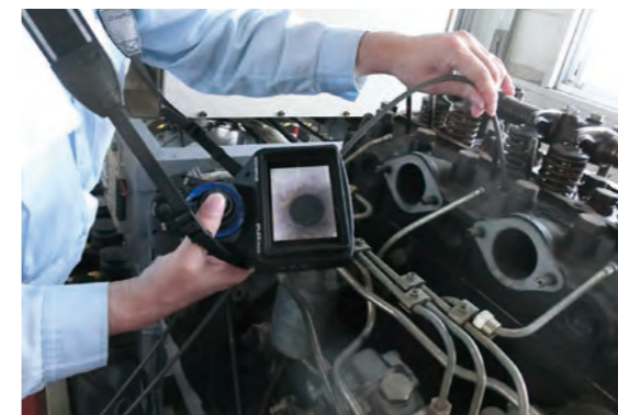
Inspection inside an engine cylinder inside
