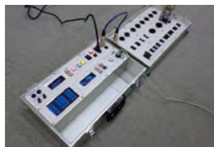
Contact resistance tester for auxiliary relays
