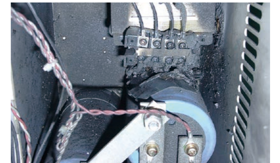
Burning of a electrolytic capacitor in the main circuit of an inverter (parts life)
