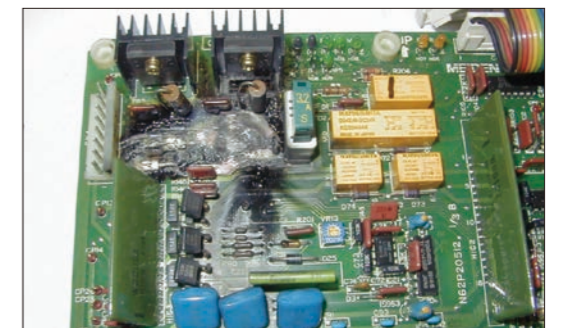
Burning of a printed circuit board (capacitor leakage)
