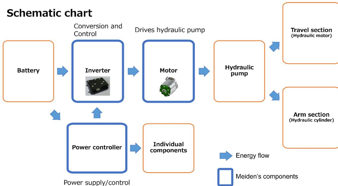
Mini excavators are conventionally used in urban areas and indoors. This requires improved working environments and anti-noise measures. Changing the power source from an engine to a motor not only reduces the environmental impact by eliminating emissions of gas and heat, but also has the advantage of reduced noise levels.
