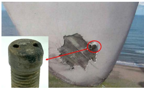
An example of damages done to a receptor and blade after a lightning strike.
