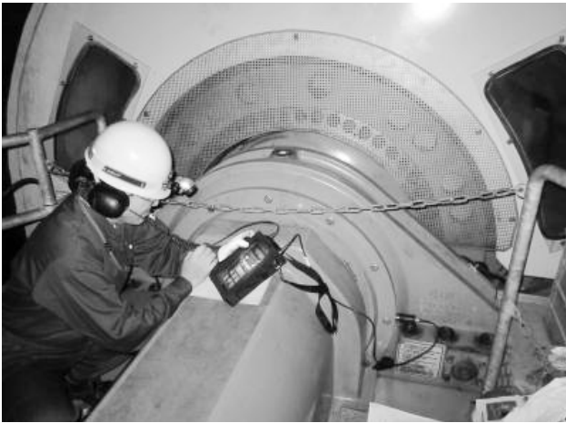
Fig. 4 Bearing Deterioration Diagnosis
