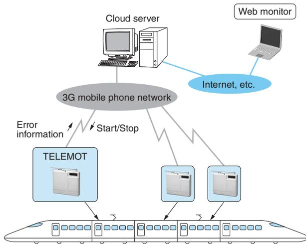
**Fig. 16** Outline System Configuration for Remote Operation
