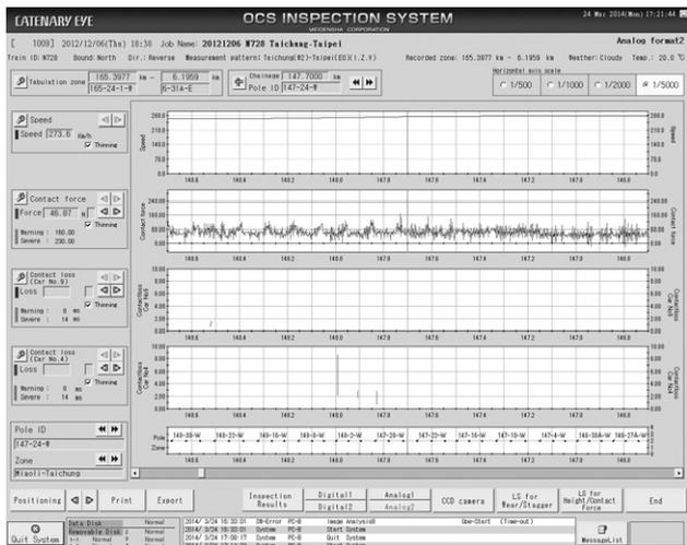
**Fig. 13** Result of Contact Force Measurement (Chart Graph)
