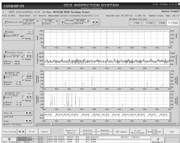
**Fig. 14** Result of Contact Loss Measurement (Chart Graph)
