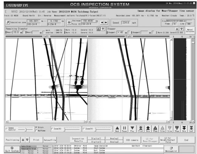
**Fig. 12** Example of Wearing Surface Image during Daytime Inspection
