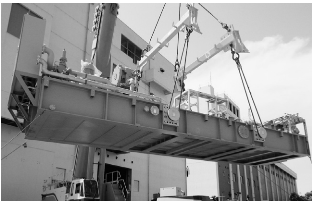
Fig. 3 Mounting Frame when Engine was Unloaded
