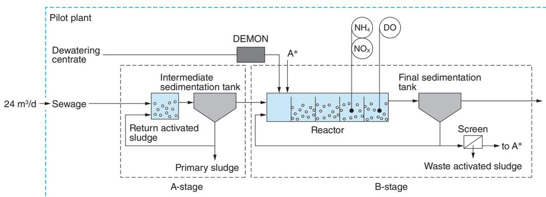
**Fig. 6** Processing Flow of Pilot Plant
