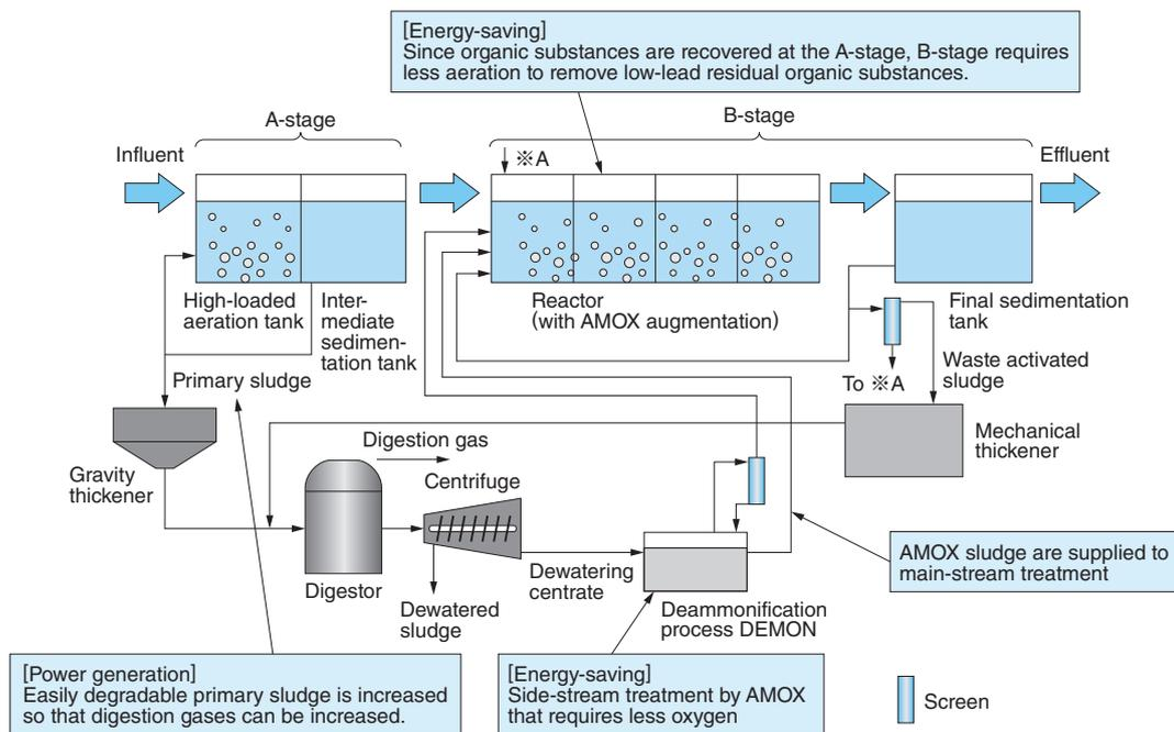
Fig. 5 Conceptual Diagram for Combination of AB Process and DEMON
