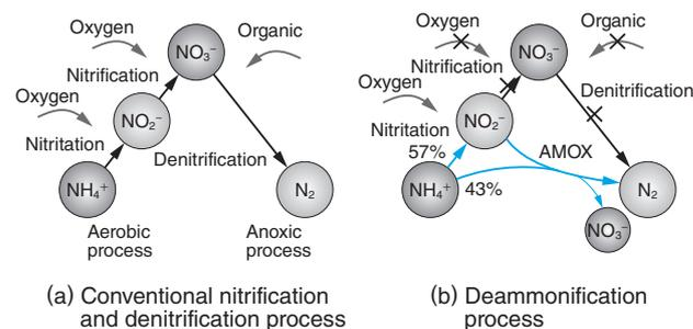
**Fig. 1 Comparison between Nitrification and Denitrification Process and Deammonification Process**
