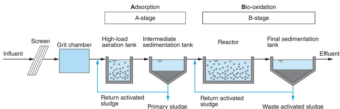
Fig. 3 Flowchart of AB Process
