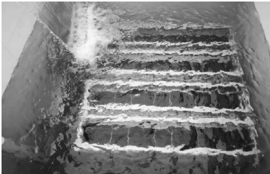
Fig. 9 Ceramic Flat Sheet Membrane Unit for Water Purification Facilities in China
