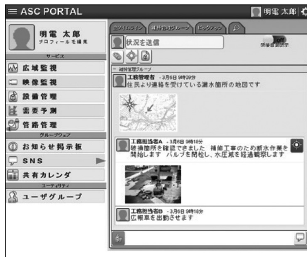
Fig. 7 Display Example of Information Sharing Screen with Maintenance Management Service Site by Using SNS Function
