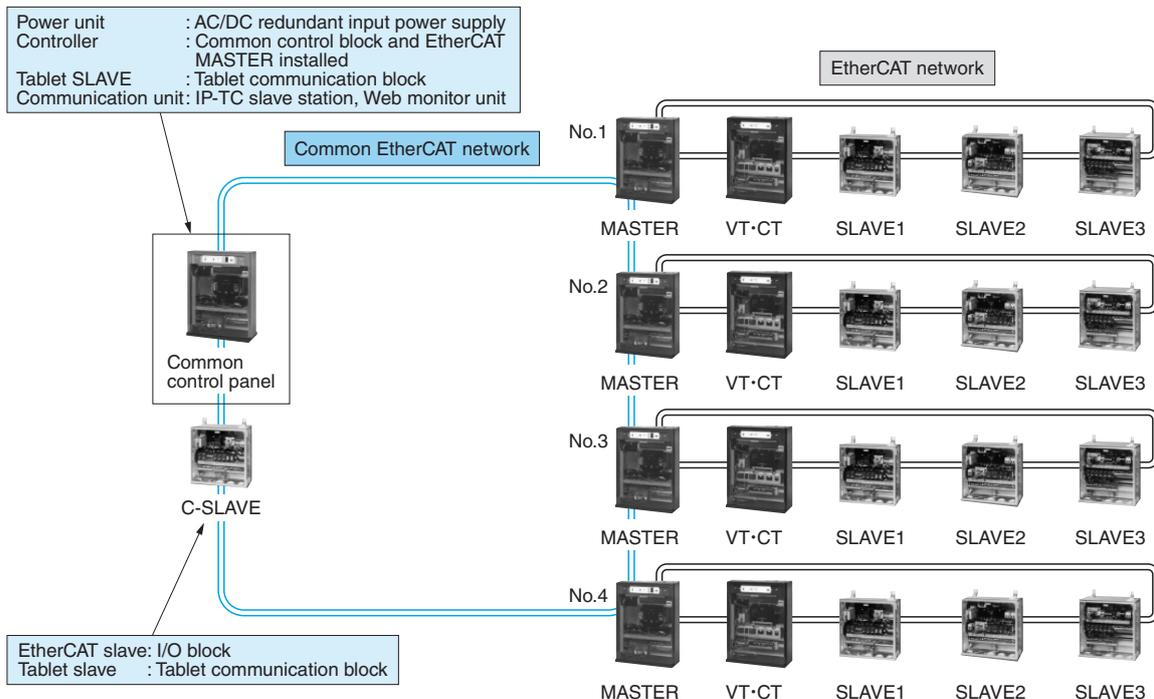
**Fig. 3 Example of Multi-Unit System Configuration**
