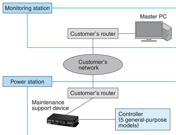
**Fig. 5** Example of Maintenance Support System Configuration
