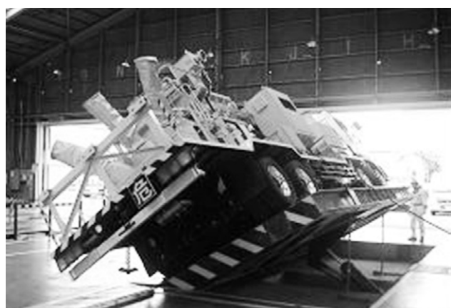
Fig. 1 View of Measuring the Maximum Inclination Angle without Tipping over a Mobile Transformer
